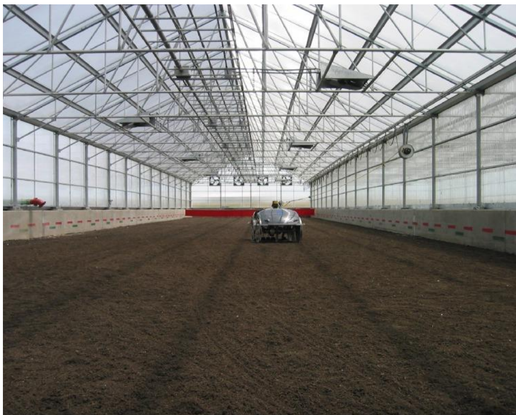
Figure 13-17. Solar dryer with electric mole
