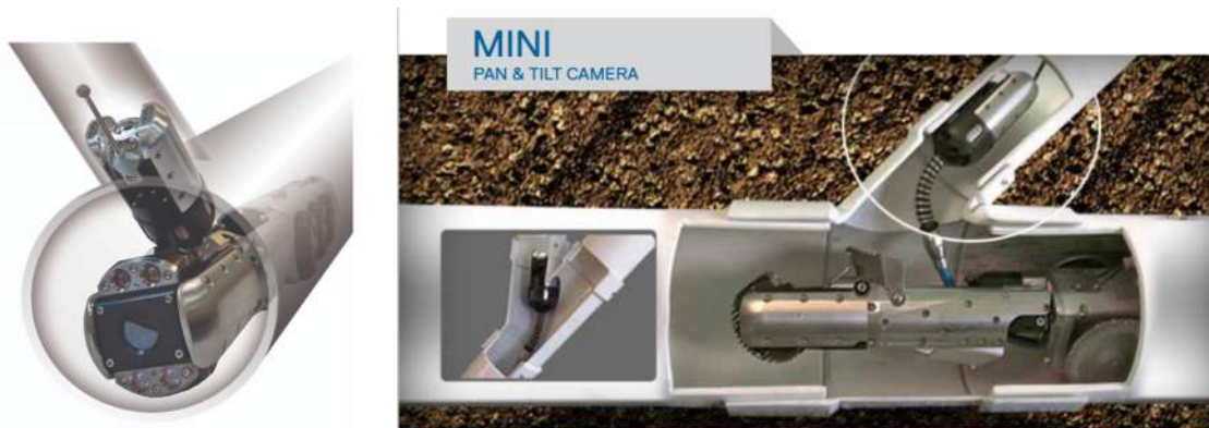
Figure 3. Robotic transporter equipped with mainline CCTV camera system.
