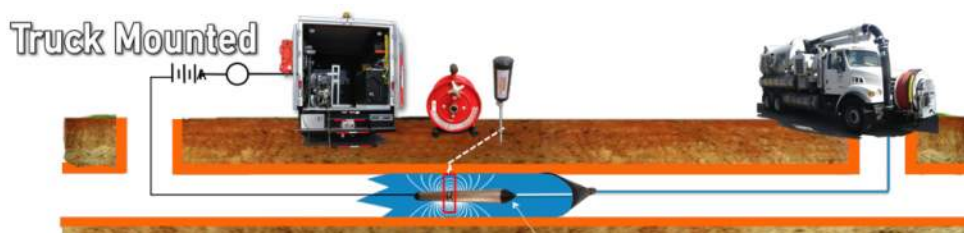
Figure 2. FELL inspection equipment setup and operation.
