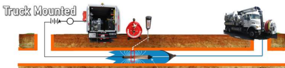
Figure 2. FELL inspection equipment setup and operation.
