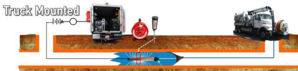
Figure 2. FELL inspection equipment setup and operation.
