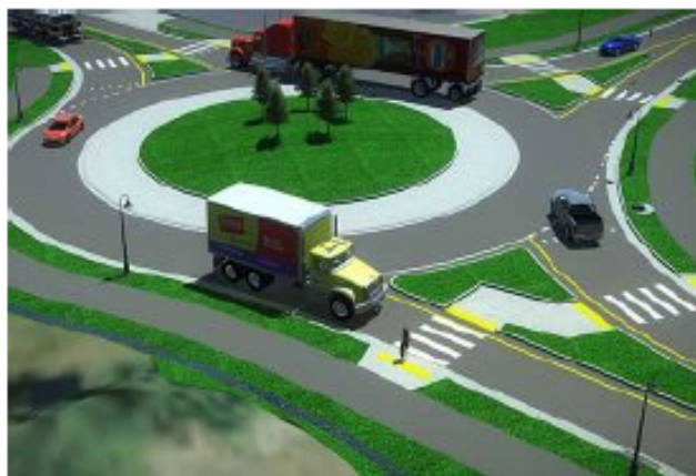
ROUNDBABOUT 3D VISUALIZATION OF A PROPOSED ROUNDBABOUT CAN BE USED TO SHOW PROPOSED ENTRY VIEWS AND ANGLES
